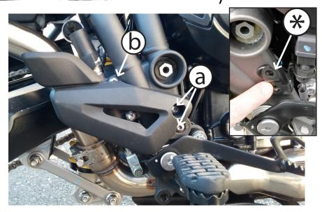
(a) Use a 5mm allen tool to Remove the (2) OEM fasteners and pull off the plastic OEM guard. (b) Once the guard is removed, the upper rear brake master cylinder bolt can be removed.
